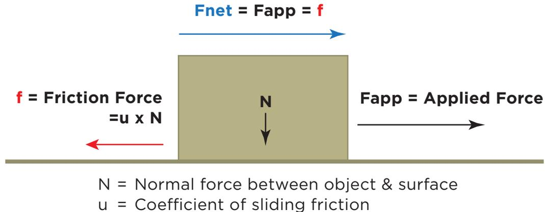
The reason we use wheels in material handling is to significantly lower effort (force) required to move an object. Imagine pushing a refrigerator or a piano without wheels! Furthermore, consider how much easier it would be to push the box (mentioned earlier) across the floor if it were on wheels.
