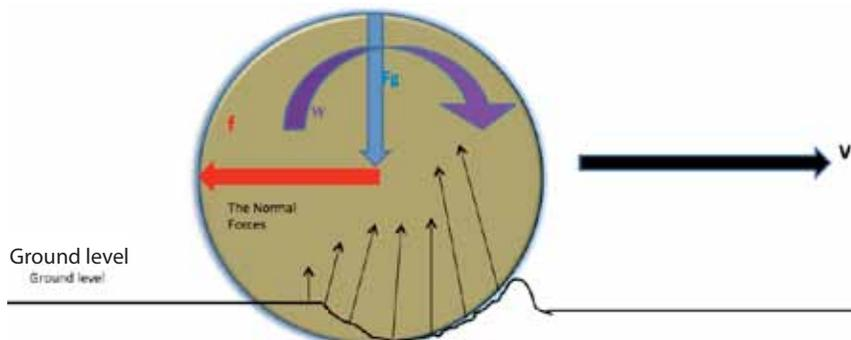
As one can see in this exaggerated view, both the wheels and the surface undergo deformation to the extent determined by the elastic properties of the two surfaces.
